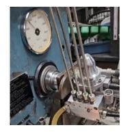
Kugelfischer mechanical injection on the test bed. Pump was used on a variety of cars from 1960s to 1980s, including various Porsche, Lancia, Ford Peugeot and BMW.
